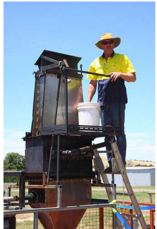
Demonstration of a Real Power Systems gassifier at the Gunning Hub
